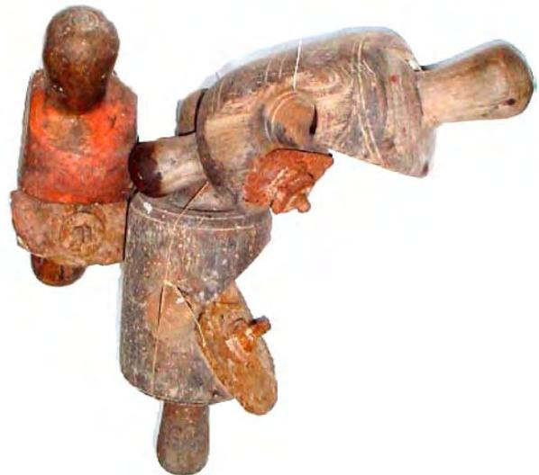
Oak **spokes** were probably also made here although we have no templates. You can see examples of rounding planes that were used to form the round tenons on the spoke ends.
