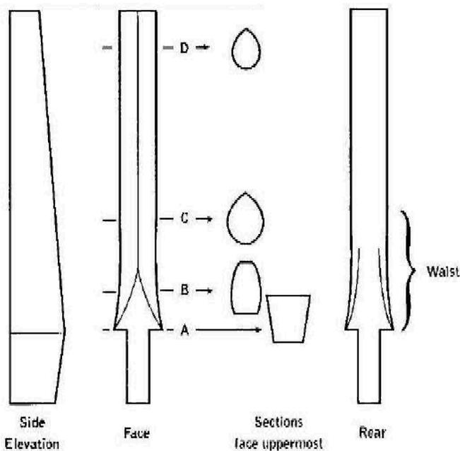
**Spokes** were shaped to provide strength and elegance to the wheel. The hub end carried a rectangular tenon and the outer end had a round (dowel) tenon to fit into the **felloes**.
