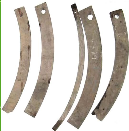
**Felloes** are the curved segments that fit together to form the rim of a wheel. You can
