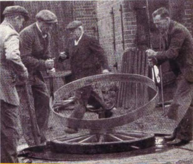
Meanwhile, the wheel was mounted on a tying platform - usually a large stone or metal plate - using a clamp to hold the hub of the wheel.
