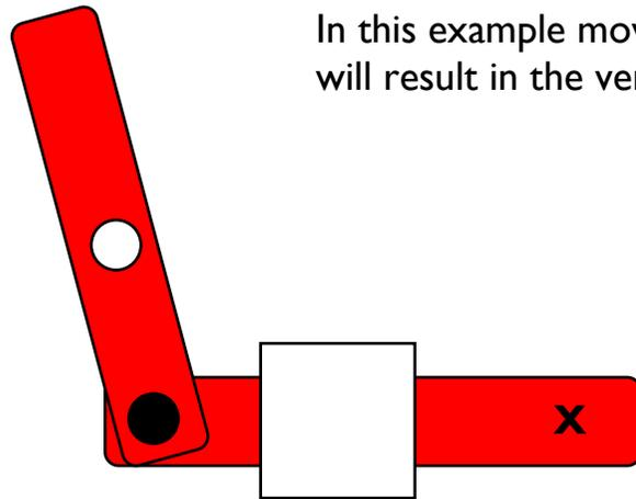
In this example moving the horizontal bar will result in the vertical bar partly rotating
