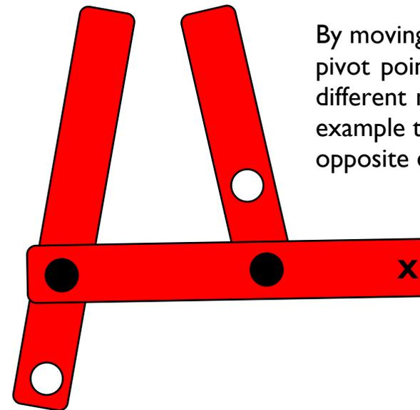
By moving the fixed and loose pivot points you can achieve different movements. In this example the two levers work in opposite directions.
