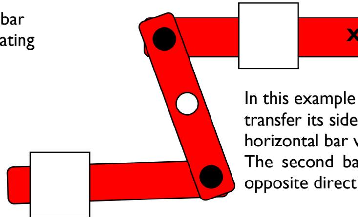
In this example the higher horizontal bar will transfer its sideways movement to the lower horizontal bar via the centrally pivoted link. The second bar will always move in the opposite direction to the first bar.
