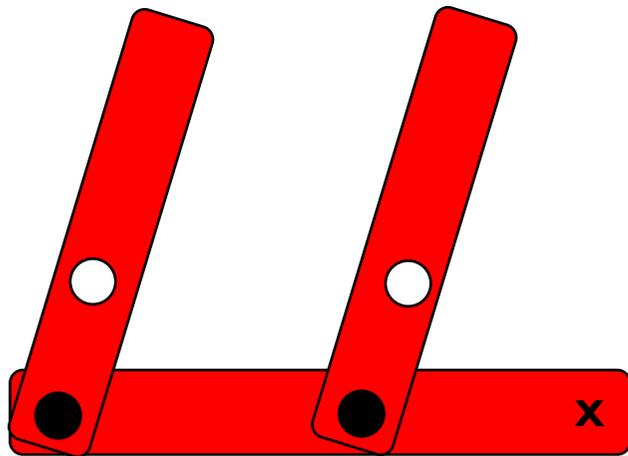
This double lever shows that one action can result in two similar reactions happening at the same time. This example is just two of the first levers fixed together.
