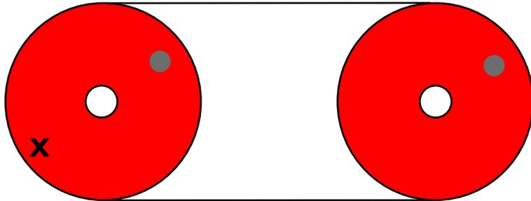
1. One pulley will drive a second pulley in the same direction
