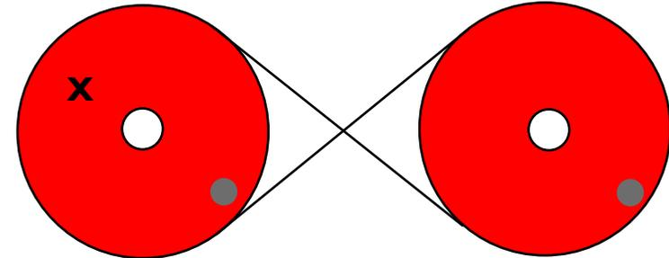
3. If the drive band is twisted the driven pulley will rotate in the opposite direction.
