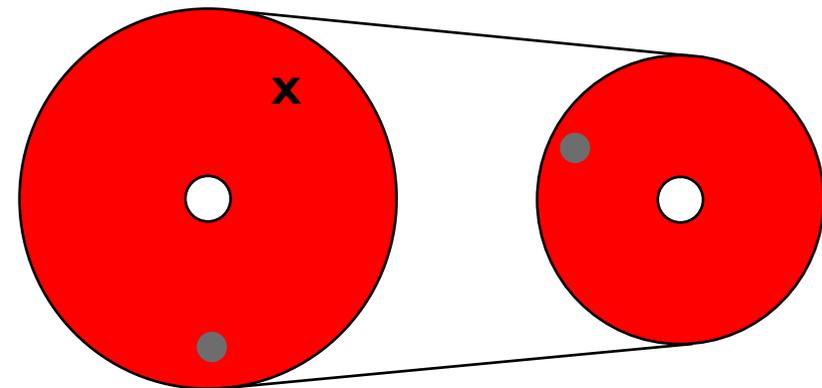
5. A larger pulley will make a smaller pulley rotate faster.
